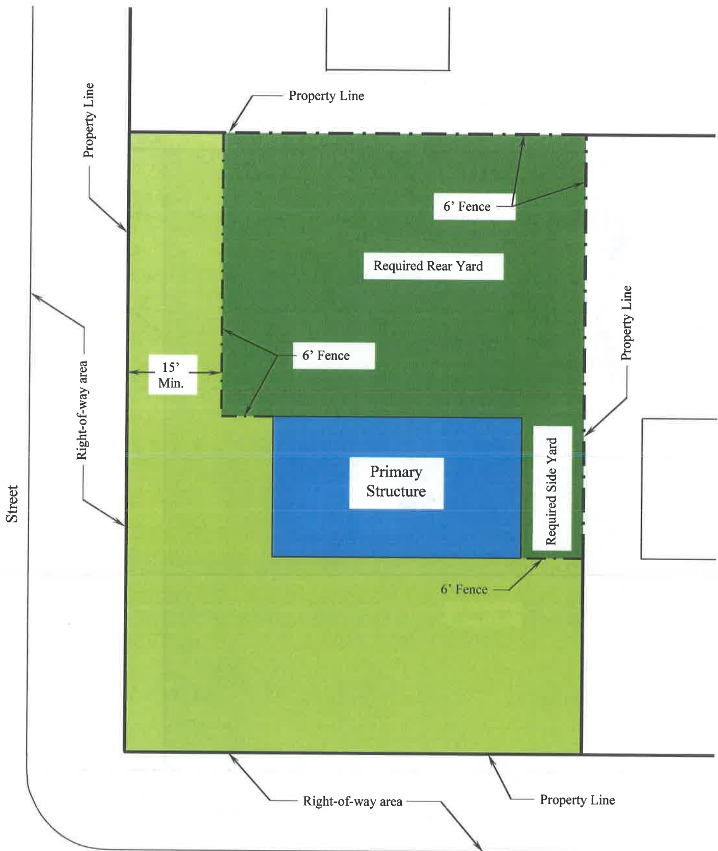
FIGURE FW2500.4 REQUIRED SIDE AND REAR YARD FOR CORNER LOT (PARALLEL)
