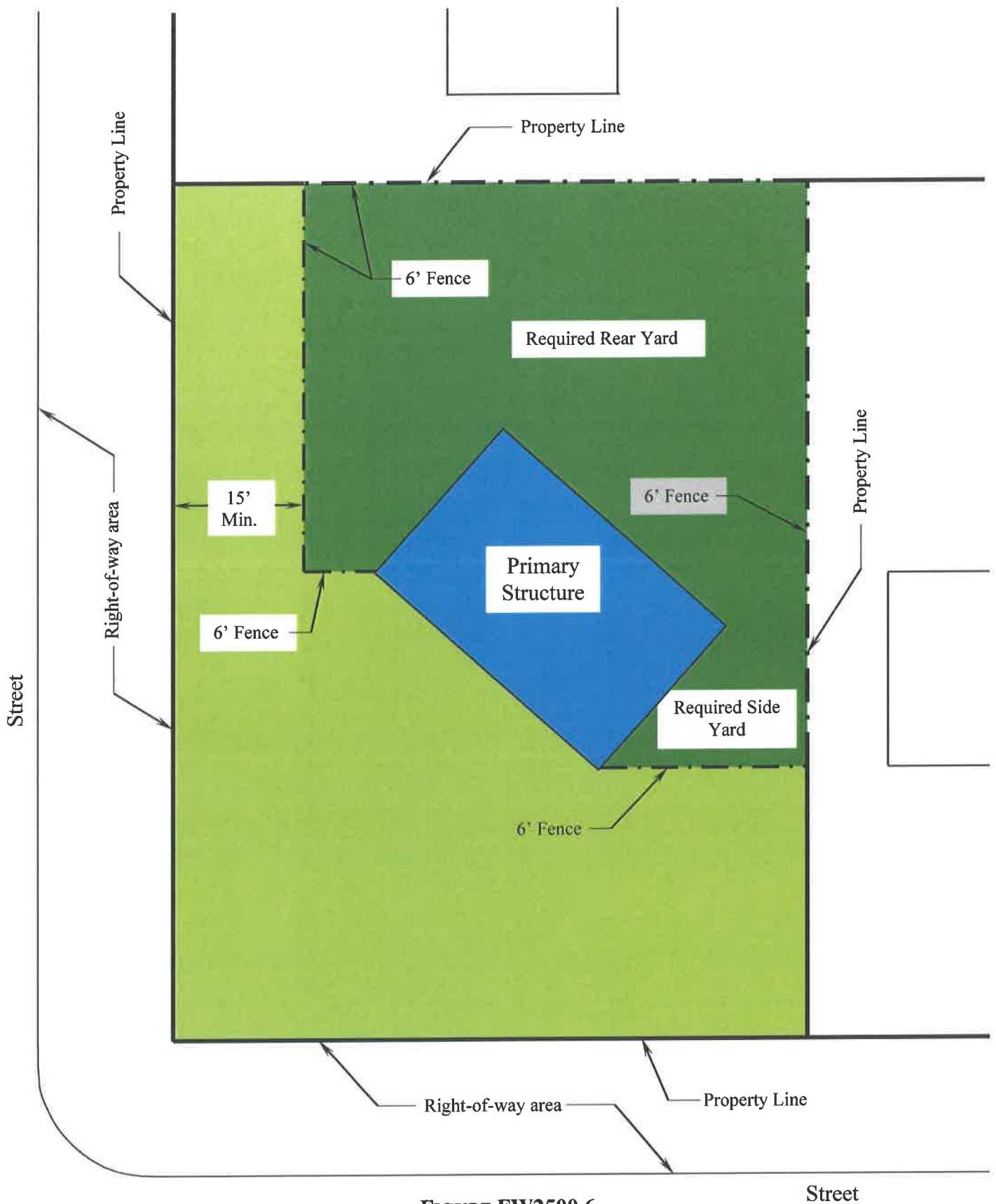
FIGURE FW2500.6 REQUIRED SIDE REAR YARD FOR CORNER LOT (ANGLE)
