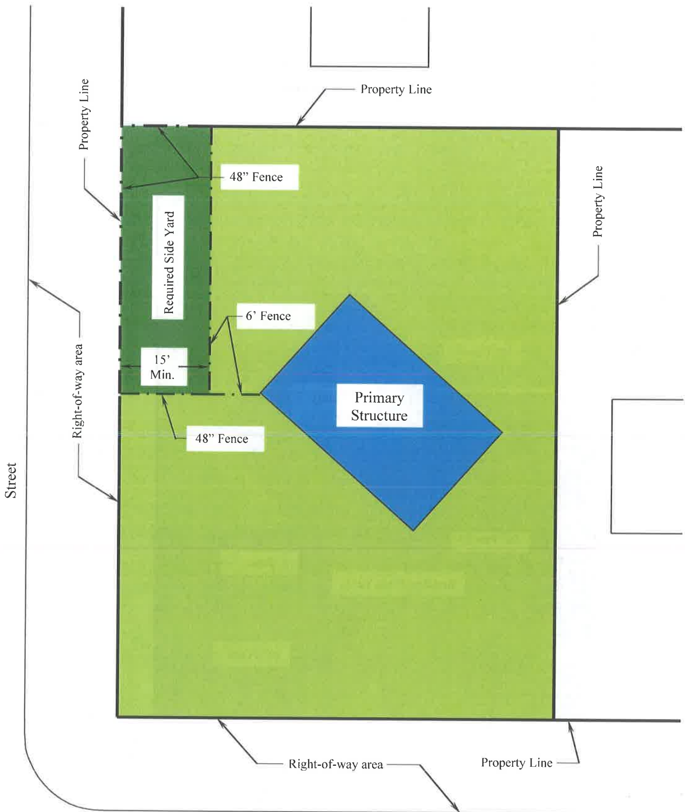
FIGURE FW2500.5A REQUIRED SIDE YARD (ADJACENT TO STREET) CORNER LOT (ANGLE)
