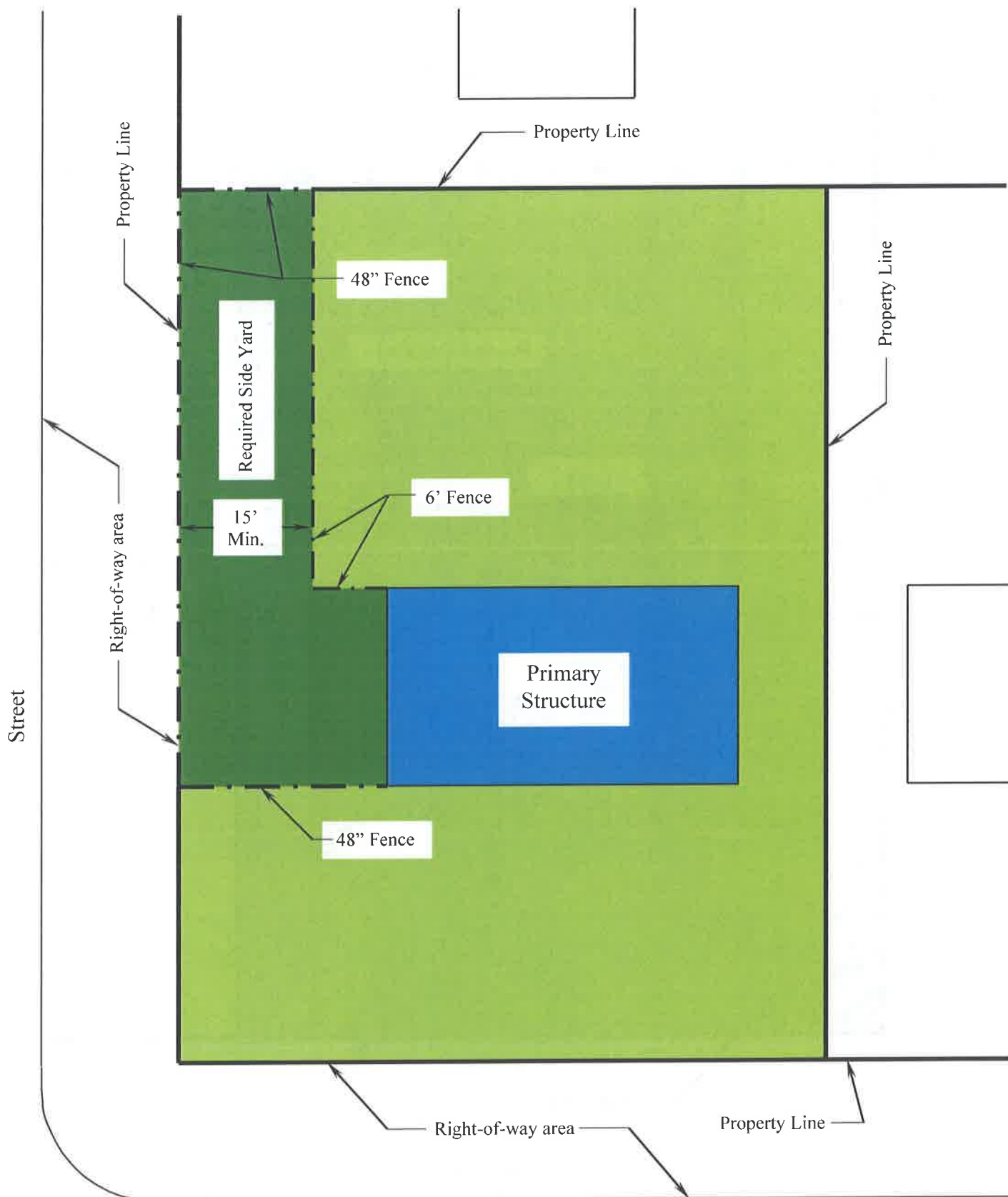
FIGURE FW2500.3A REQUIRED SIDE YARD (ADJACENT TO STREET) CORNER LOT (PARALLEL)
