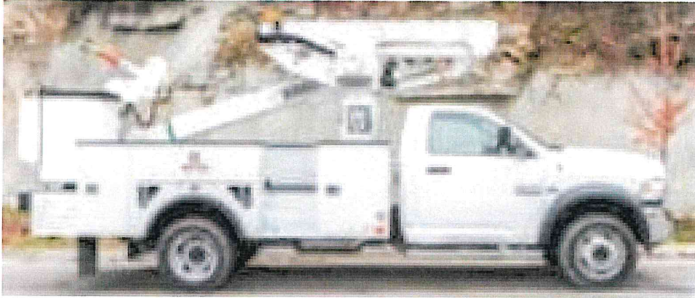
Versalift VST-40-MHI Aerial Lift on Ram 5500 Truck Chassis
